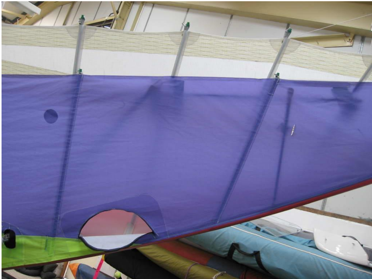
Rigging stage 12 – correct positioning of washout rods.
